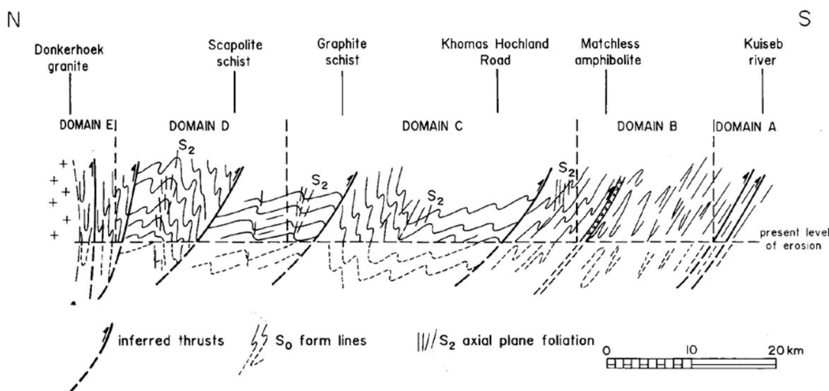
Fig. 5: Structural profile across the western Khomas Trough showing  $s_0$  form lines,  $D_2$  fabric and inferred thrust zones. Domain boundaries are based on changes in fabric development. Notice the progressive steepening of the  $s_2$  axial planes northwards.
